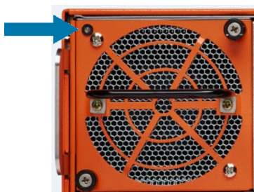
Figure 6 Individual Fan LED Location on GigaVUE-HC3 Rear
