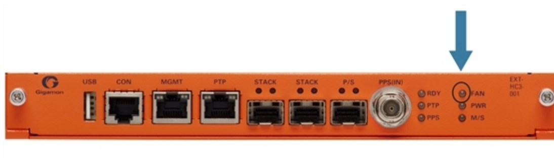
Figure 5 Global Fan LED Location on GigaVUE-HC3 Front
